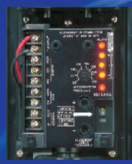
LED Level Meter for Beam Alignment Three LEDs on the receiver act as a Level Meter to visually display the beam reception level. Each LED flashes and then turns off in order as the detector is aligned. This user-friendly feature allows anyone to perform quick alignment.
